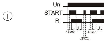
Deactivation and activation lags with support function enabled. If the START voltage is supplied for less than 45sec., it is ignored by the system, however if it is longer, the relay is activated after the 45sec and the preset time value is counted down with the trailing edge of the START signal. If another START impulse is applied during the countdown, then the trailing edge of this signal will result in the repeated countdown sequence (e.g. for ventilation purposes: short activation of the lighting does not turn the fan on, but if the lighting is activated for longer than the 45sec, the fan will start).
